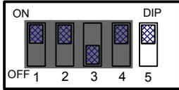
Switch 5 ON for a 17 minute run-time.
